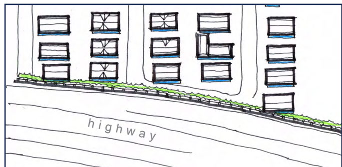
Figure 44: A wall barrier with vegetation, shown in plan, running along the highway and protecting the existing residential neighborhood. Currently there is no barrier along this section of I-93.
