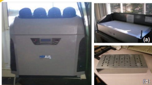
Figure 1. HEPAiRx room air purification system (Air Innovations) used in the study with a) HEPA and b) Sham filter.
