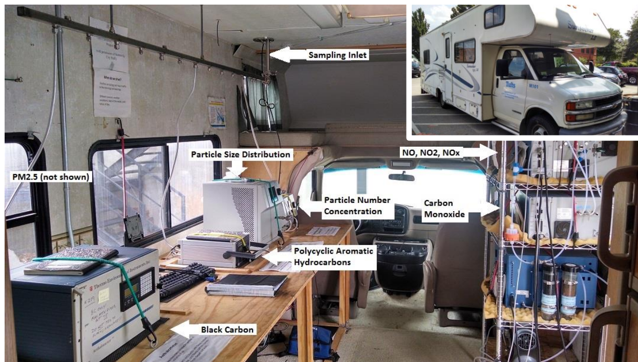
Figure 1: Air monitoring equipment setup inside TAPL.
